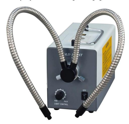
ACUCAL Fiber Cold Light Illuminator refers to an illuminating light source that does not contain or contains less spectrum of infrared heat radiation in a illuminating or light guiding body. In Optical Fiber Cold Light Source, after the illumination beam is transmitted through the optical light body, the heat radiation is not brought to the light exit port, hereby achieving "COLD LIGHT" effect.
